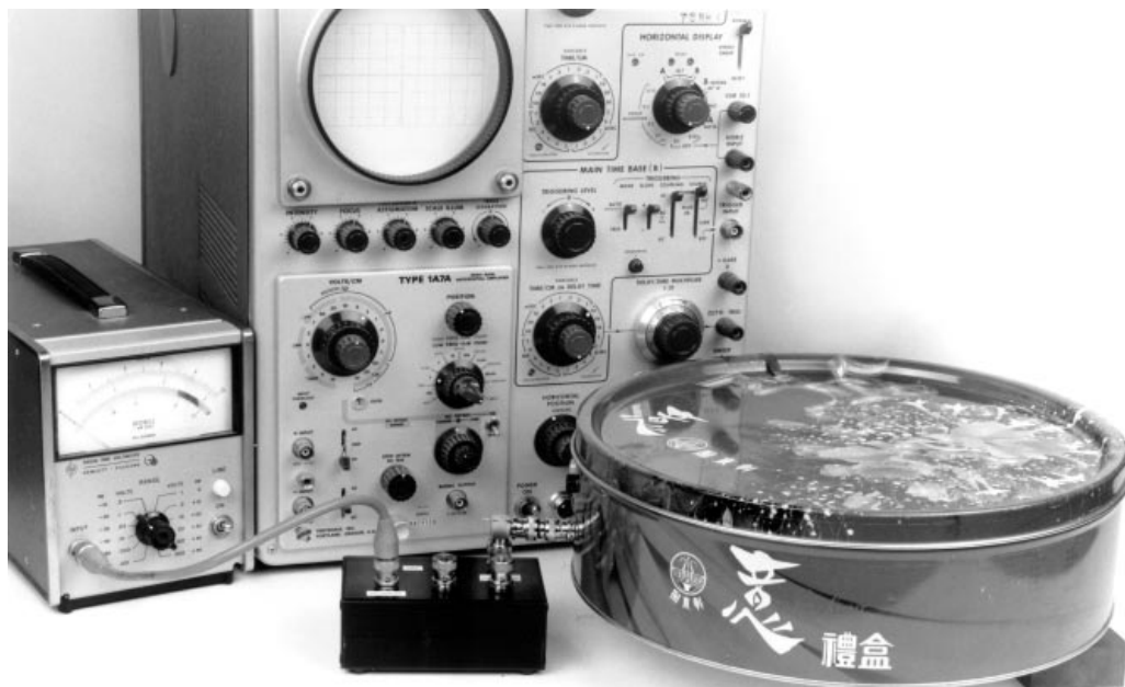
Figure 6a. LDO Noise Measurement Bench Setup. Shielded Can Contains Regulator; Noise Filter Circuitry Occupies Box at Photo Lower Center. Oscilloscope and RMS Voltmeter Are Not Simultaneously Connected, Precluding Ground Loop from Corrupting Measurement
